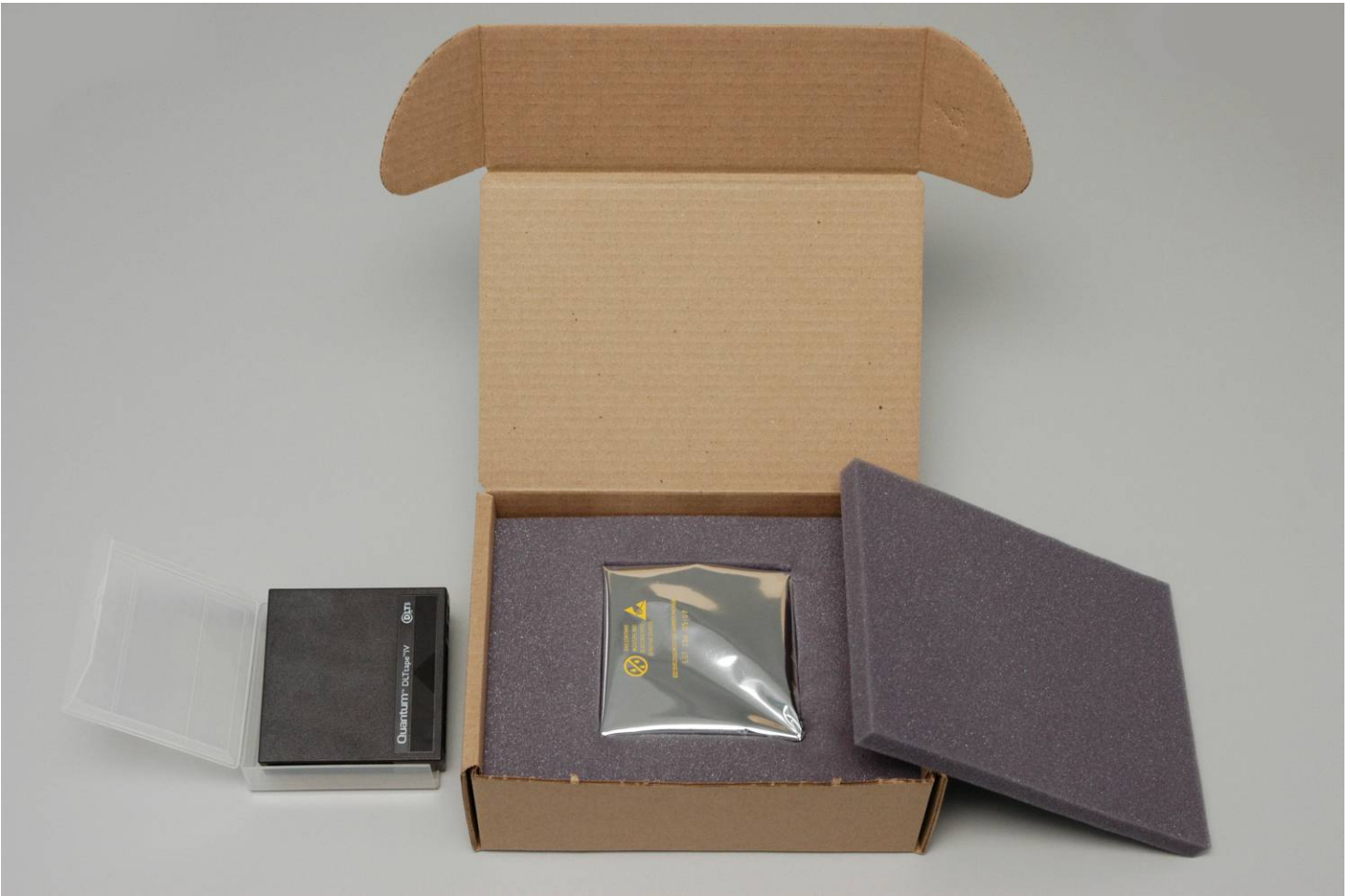
Figure 2 - DLT data cartridge with OEM container (left), static bag sealed cartridge in recommended foam / cardboard container (right).
